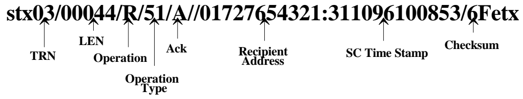
Figure 2.2 Example of a Submit Short Message operation ACK
